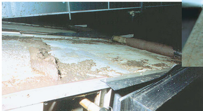
Fig. 1. Concentrated sludge accumulates on the the revolving fabric of the belt filter.
