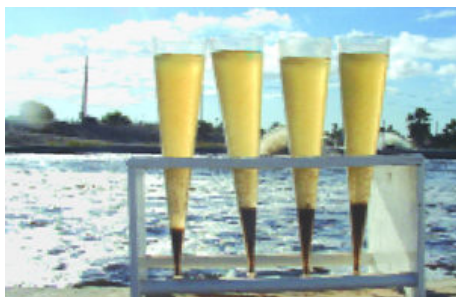
Floc volume for the active suspension pond was determined with sedimentation cones.
