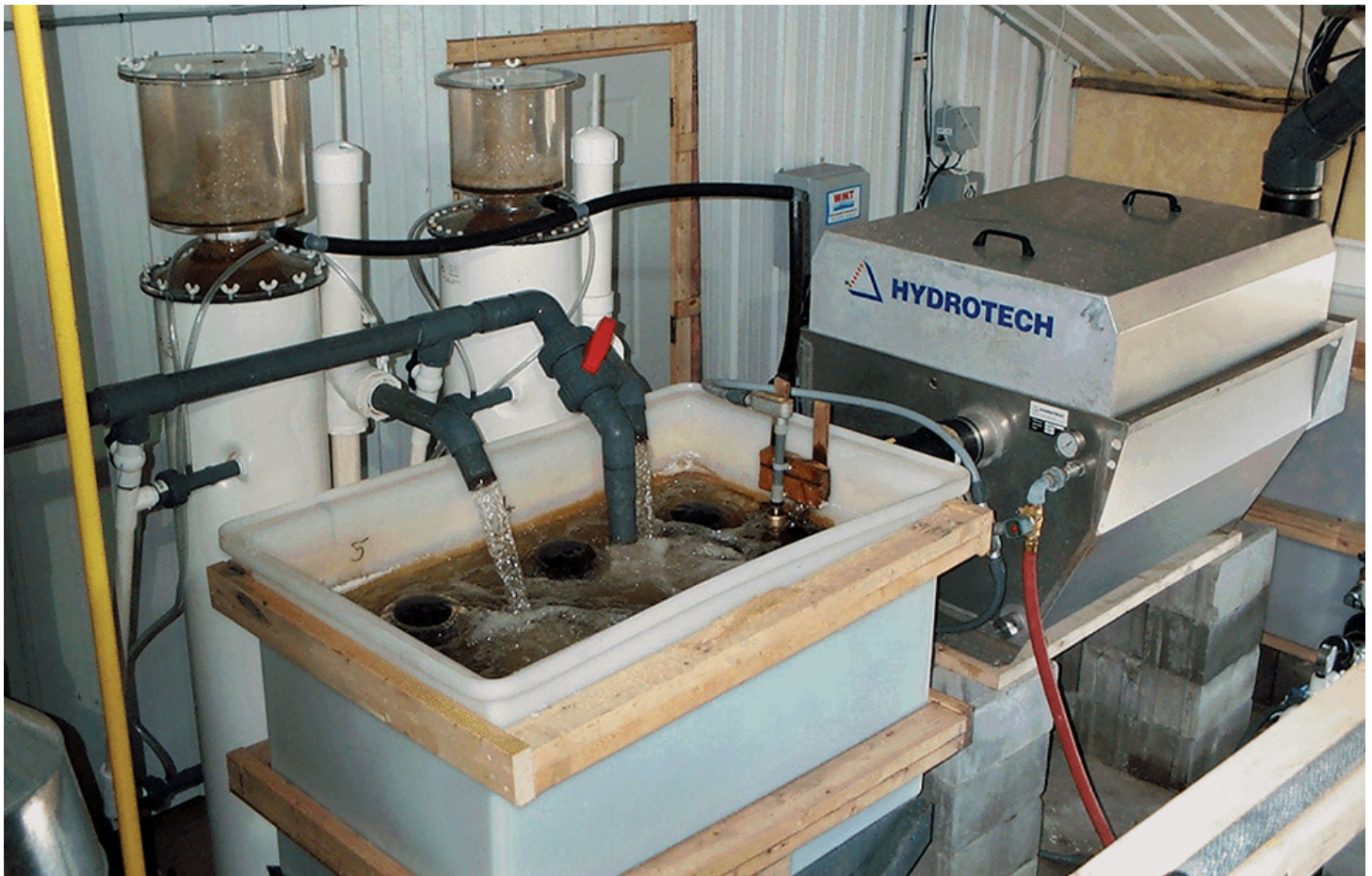
Water that drains from the culture tanks is passed through a drum filter (right), foam fractionators (columns in rear) and heating tank (foreground) before reuse.
