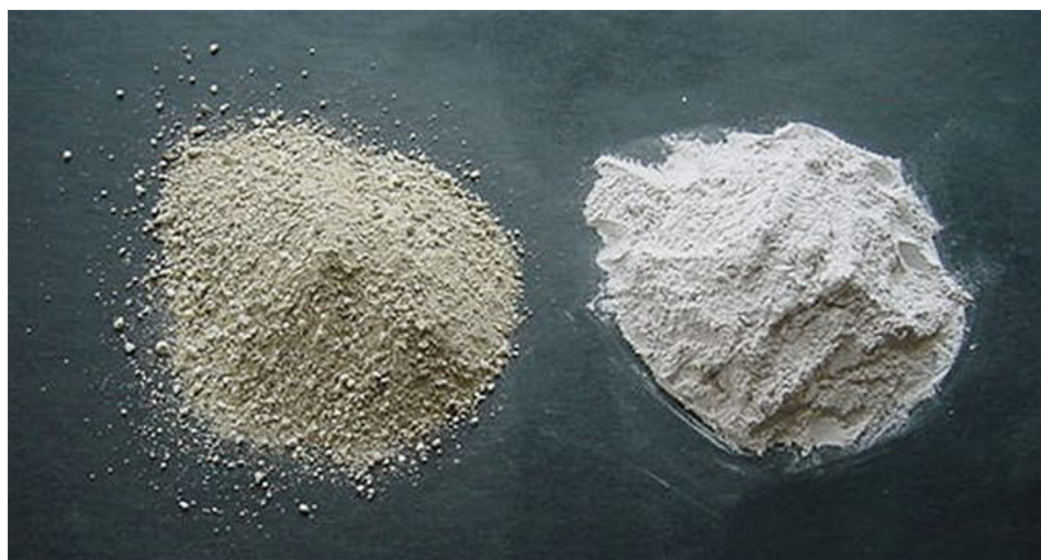
Coarsely pulverized (left) vs. finely pulverized (right) agricultural limestone. Finer limestone dissolves much faster than coarser limestone.
