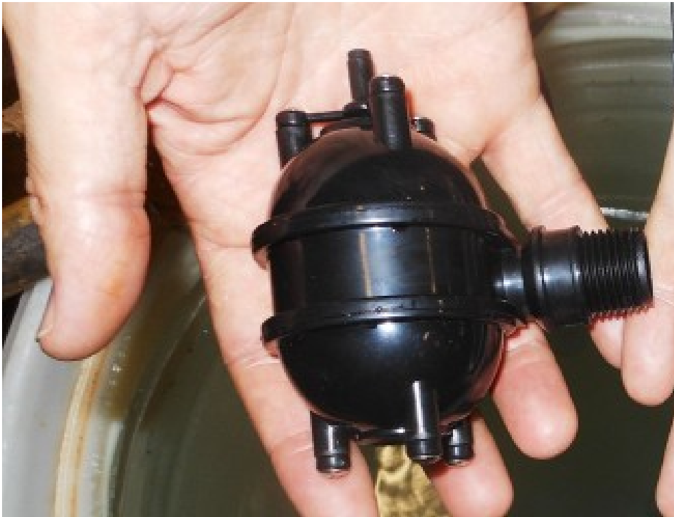
The micro-nanobubble generating device that was used in the experiment.
