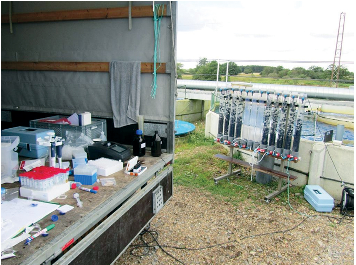
Easily degradable peroxyacetic acid residuals require immediate measurements, here with a simple mobile lab. The column set-up on the right is used to assess nitrification performance on biofilter elements exposed to disinfectant residuals.
