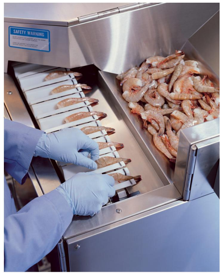
After manual loading of individual shrimp, machine peelers remove the shells and segregate them from the shrimp.
