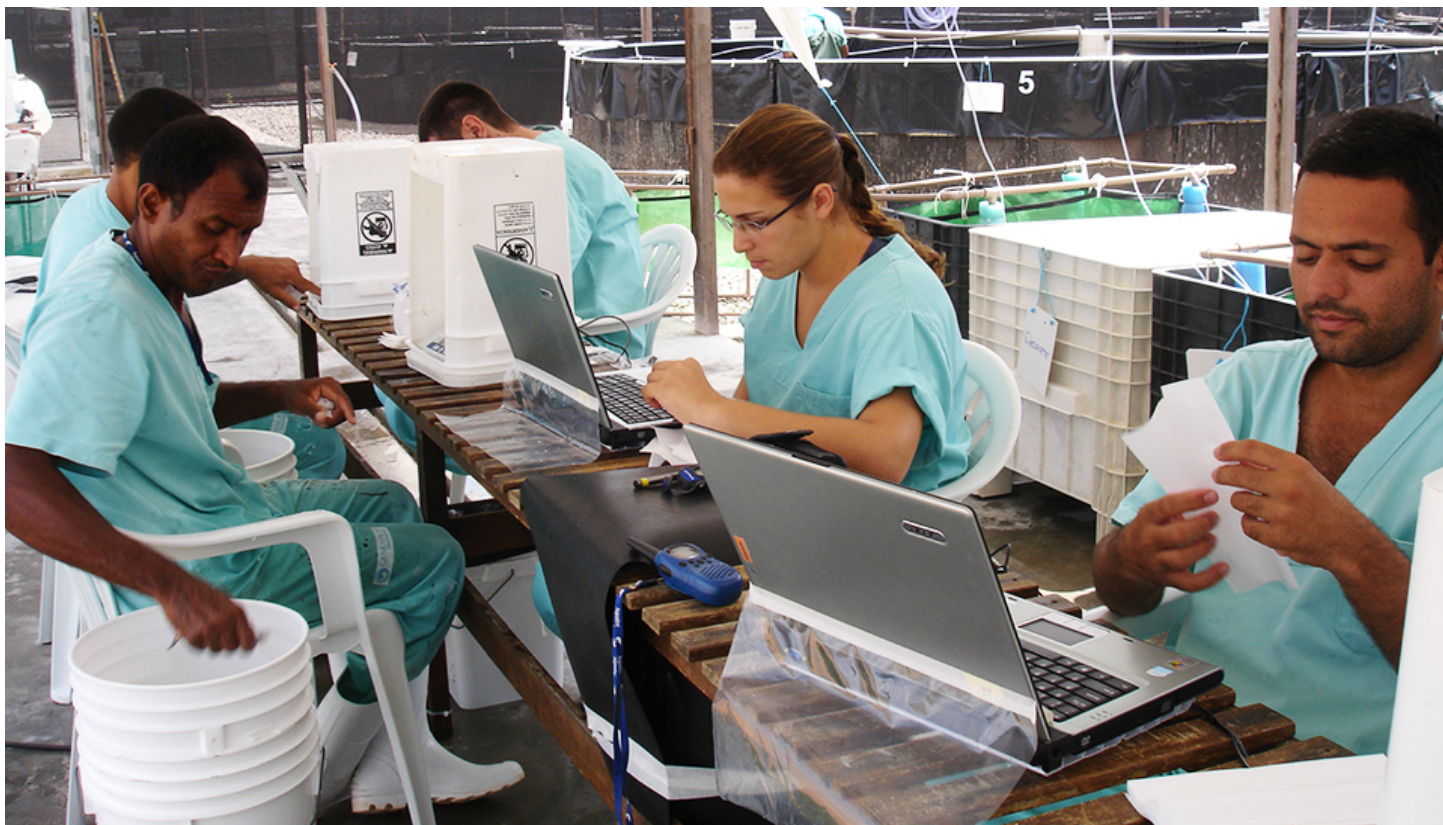
Technicians weighed shrimp during tests using electronic balances connected to computers that recorded data automatically.
