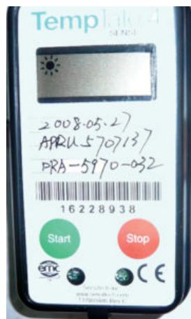
A typical temperature-recording device used in shipping containers. Photo courtesy of Sensitech Corp.
