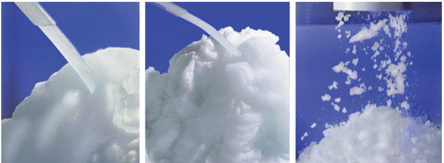
Variable-state ice slurry systems can generate product of varied consistency by controlling both the ice fraction and salinity of the discharged slurry.
