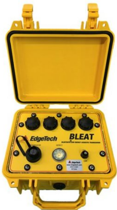
The EdgeTech apparatus includes a deck unit containing a transmitter that receives responses from the underwater unit. Photo courtesy of EdgeTech.
