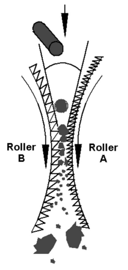
Fig. 2: Crumbler rollers rotate at different speeds and have different corrugations.
