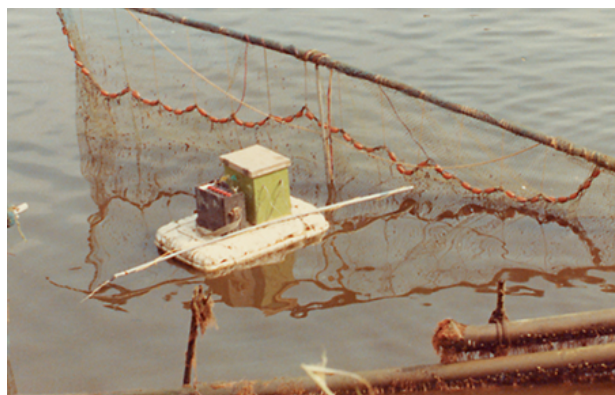
The horizontal pole of this electrical seine setup is used to spread and pull the net. The floating battery provides a weak current to stimulate burrowed shrimp to jump into the net.
