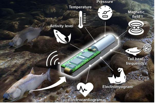
Lab-on-a-Fish is an implantable biotelemetric fish fitness tracker that uses multiple sensors to wirelessly track health and behavior.
