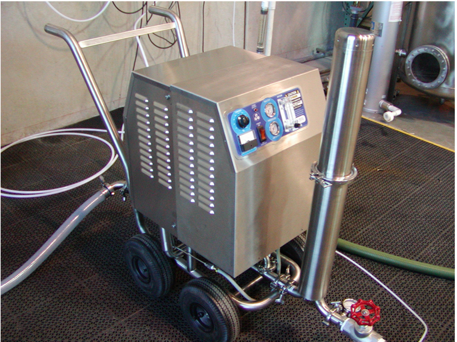
This portable ozone machine is connected to a water supply to provide ozonated water for surface sanitation and disinfection in a mobile system. Photo courtesy of Pacific Ozone Technology.
