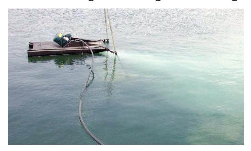
Oxygen injection systems output high-purity oxygen directly into pond water. With source oxygen fed through a hose, this floating unit
