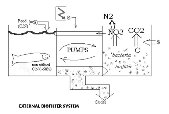
Fig. 1: Scheme of a conventional recirculation system with an external biofilter. Separate grow-out unit (left) and biofilter (right hand-side).
