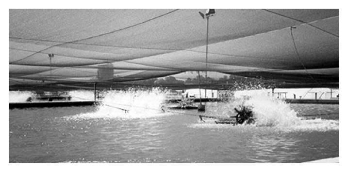
Shade cloth covering activated suspension tank to reduce algal activity and accelerate bacterial growth.
