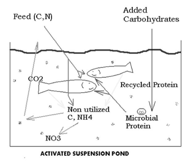
Fig. 2: Scheme of an activated suspension pond (ASP). Grow-out and water treatment take place in the same unit.
