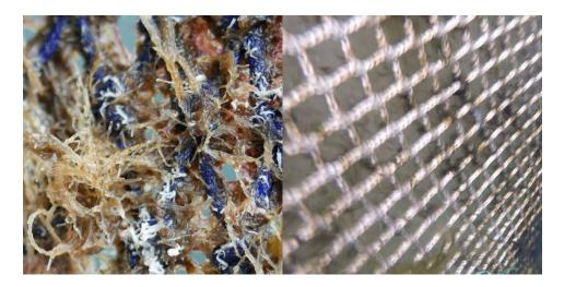
New aquaculture nets with copper ions (right) increase the material density and reduce biofouling (left), the removal of which is costly and time consuming. The metallic particles lead to a continuous release of a small amount of copper ions into the water, reducing environmental harm. Photo courtesy of Garware Technical Fibres Ltd.
