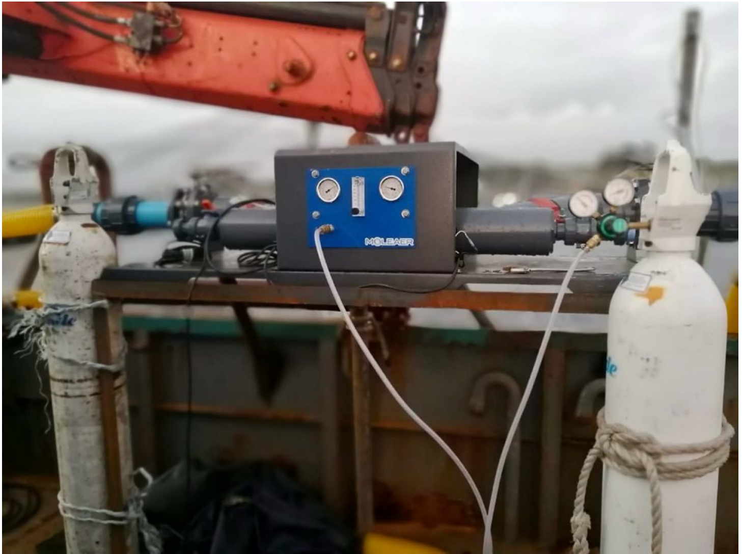
Nanobubble technology for oxygenation can improve water quality and reduce energy costs. Photo courtesy of Moleaer.
