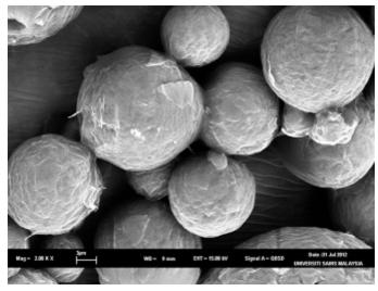
A scanning electron micrograph of the microencapsulated organic acids blend manufactured using centrifugal cool-spraying technology by Sunzen Feedtech Pte. Ltd. (Malaysia).
