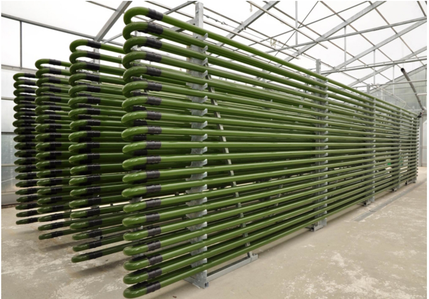
A tubular glass photo-bioreactor for the cultivation of microalgae and other photosynthetic organisms. It has an operational volume of 4,000 liters and the principle was developed in the late 1990s.
