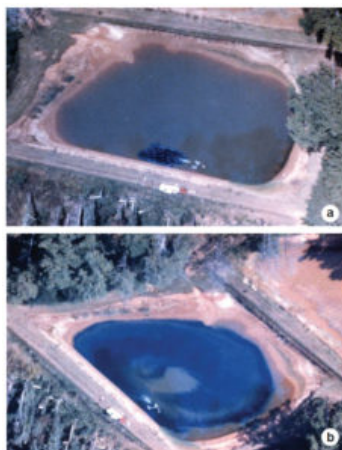
Fig. 1: Surface water circulation testing. Blue dye was applied at an aerator in this test pond (a). Most of the pond appeared blue after 20 minutes (b).
