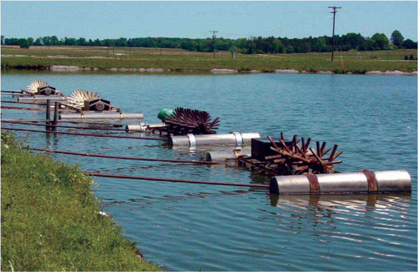
Increased aeration can improve catfish yields by raising dissolved oxygen concentrations in the water.
