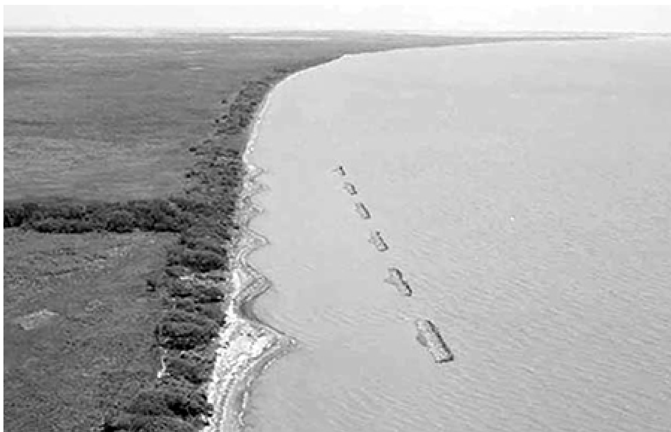
A classic tombolo effect, often seen with breakwaters of this kind, caused the salient to form directly behind the breakwaters on the shoreline at a demonstration project in Vermilion Parish, Louisiana. Photo courtesy of USDA-NRCS.
