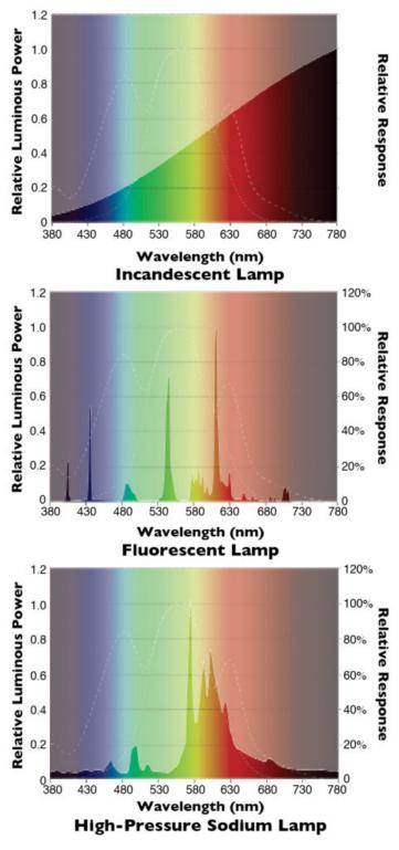
In general, incandescent bulbs emit light with predominantly red wavelengths. Compact fluorescent lamps emit in the blue/green wavelengths, and high-pressure sodium lamps emit in the yellow/green wavelengths.
