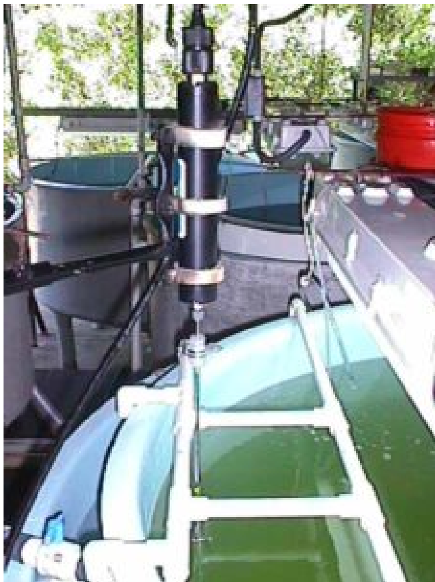
A Doppler current meter measured turbulence in the larval tanks
