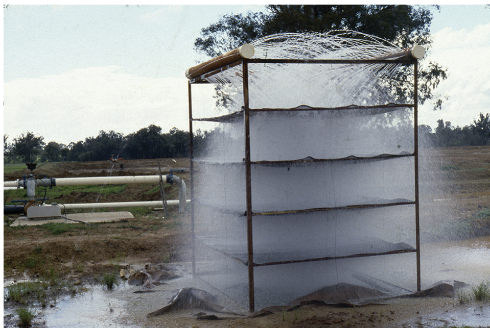
Well water that contains higher concentrations of ferrous iron can be treated by gravity aeration.
