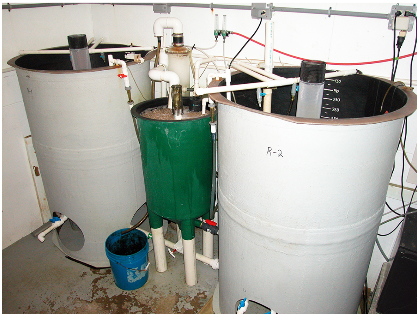
Rotifers are produced in an automated generator comprised of two 500-L culture tanks, a fluidized-bed biofilter and a protein skimmer.
