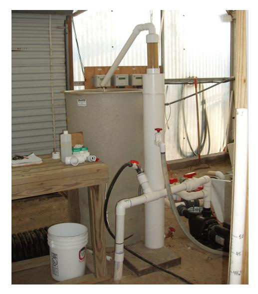
Two raceways were each outfitted with a commercial foam fractionator. Due to their ability to quickly reduce particulate load, the fractionators were only operated for a few days at a time.
