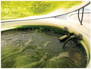
The turbidostats produce a continuous supply of high-quality algae to the hydraulically linked reactors.
