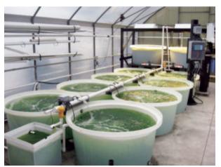
The Hydraulically Integrated Serial Turbidostat Algal Reactor consists of two turbidostats, eight CFSTRs and a control system.
