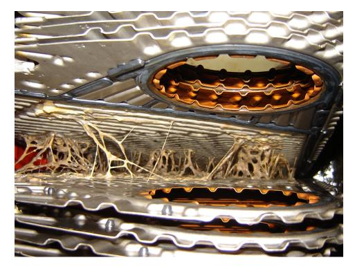
Severe biofouling of flat-plate heat exchangers can reduce efficiency to near zero.
