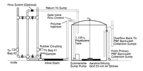
Primary treatment consisted of a sludge-holding tank, dosing pump with inline mixer for coagulation/flocculation aids and distribution/pressure equalization manifold for two geotextile bags.
