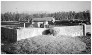
At this zero-exchange tilapia culture operation in Saudi Arabia, dried foam condensate produced by the skimmer is used to fertilize nearby trees.
