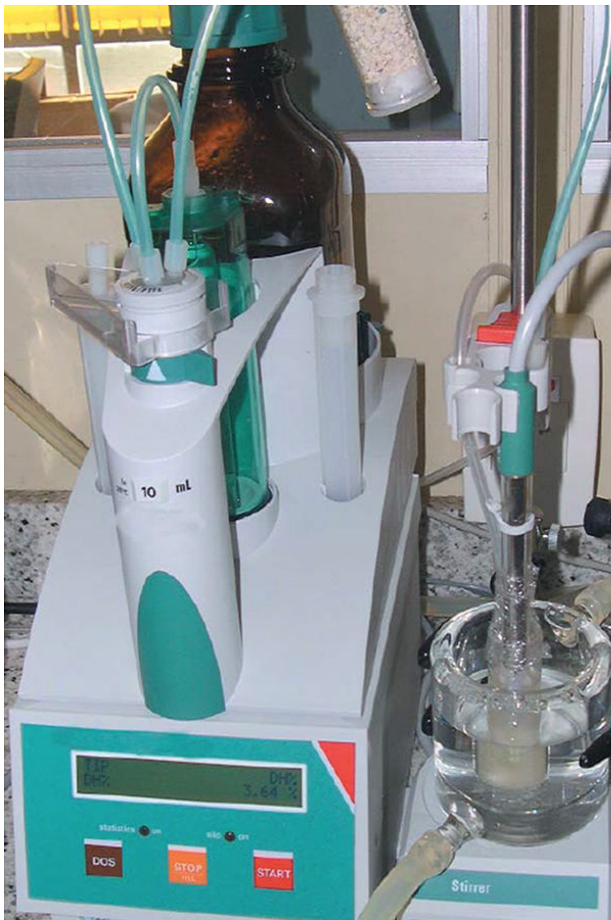
The new in vitro pH-stat assay simulates the digestion of a protein source by the enzymes of the target animal. (Photo by Daniel Lemos.)
