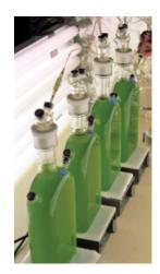
Photobioreactors like these lab-scale units are self-contained systems that continuously pump water containing algae through clear vessels of various types to expose the algae to light for growth. (Photo courtesy of the U.S. Department of Energy National Renewable Energy Laboratory.)
