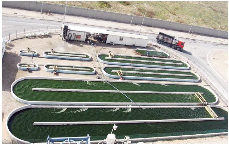
While most commercial microalgae production is done in open ponds, closed raceway systems can provide a greater degree of environmental control. (Photo courtesy of the U.S. Department of Energy National Renewable Energy Laboratory.)
