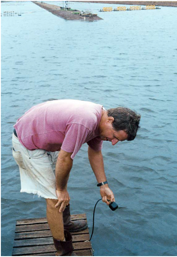
Checking continuous dissolved oxygen sensor. Note the central baffle and paddlewheels in the background.
