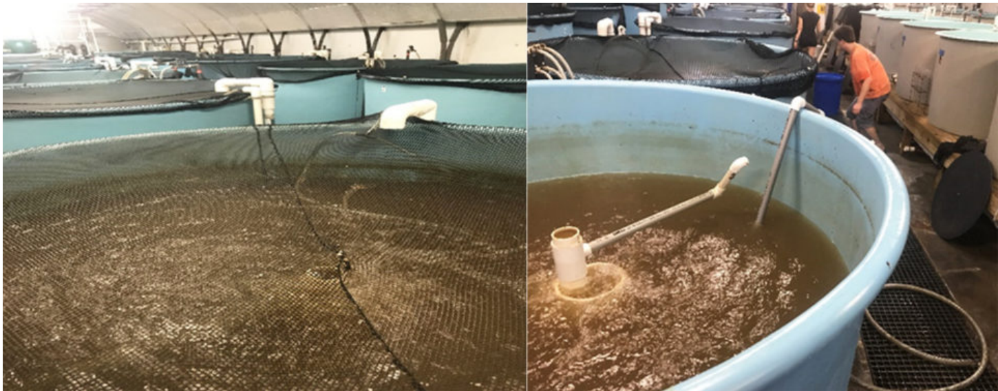
Fig. 1: Experimental 1-cubic-meter tank design. The tank on the right, partially drained, shows the airlift driven circulation system. Sixteen liters of biofloc from the FAU-HBOI Integrated Multi-Trophic Aquaculture (IMTA) ex-situ bioreactor were added to each tank three weeks prior to shrimp addition. One hundred 1.5-gram shrimp were placed into each tank on May 2, 2017. AquaStar® Growout was top dressed onto Zeigler shrimp HI-35 feed (2 mm pellets) at 0, 2, 3 or 5 g/kg (0 percent, 0.2 percent, 0.3 percent, or 0.5 percent).
