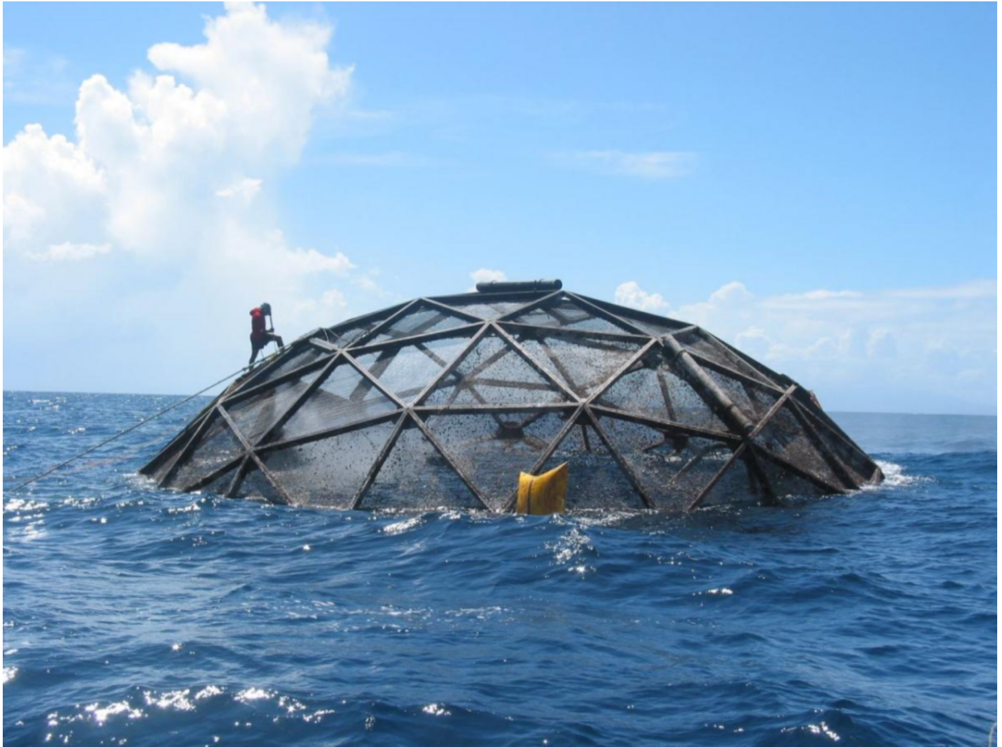
The Aquapod is a free-floating fish farm that can accommodate several hundred thousand fish. Photo courtesy of InnovaSea.
