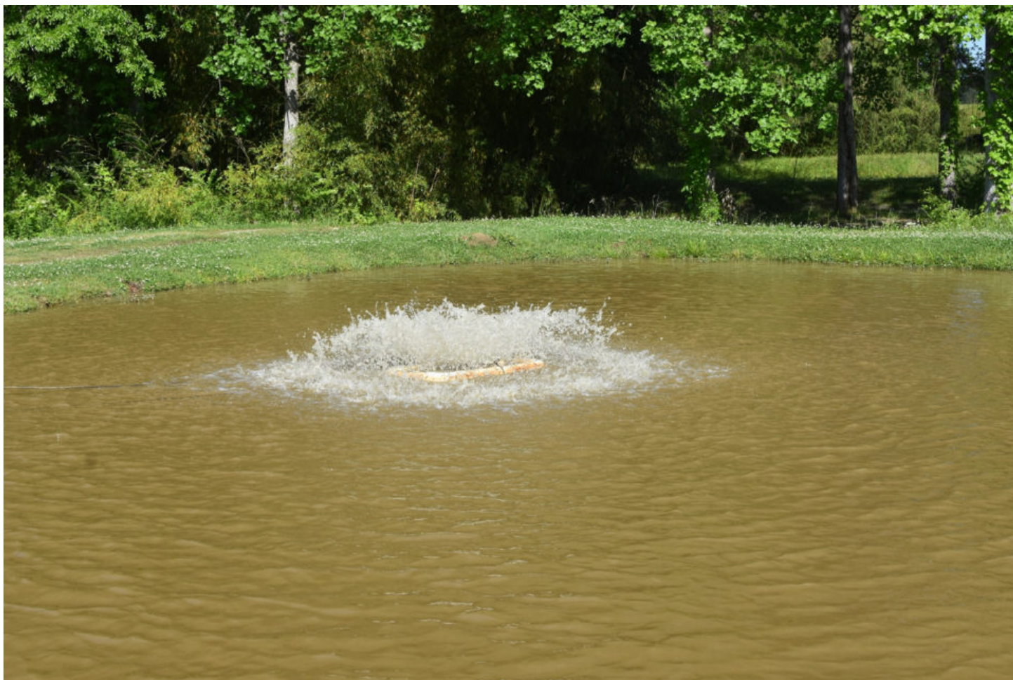
One of the 0.5-hp Air-O-lator aerators used in this study, showing water being splashed into the air during operation.
