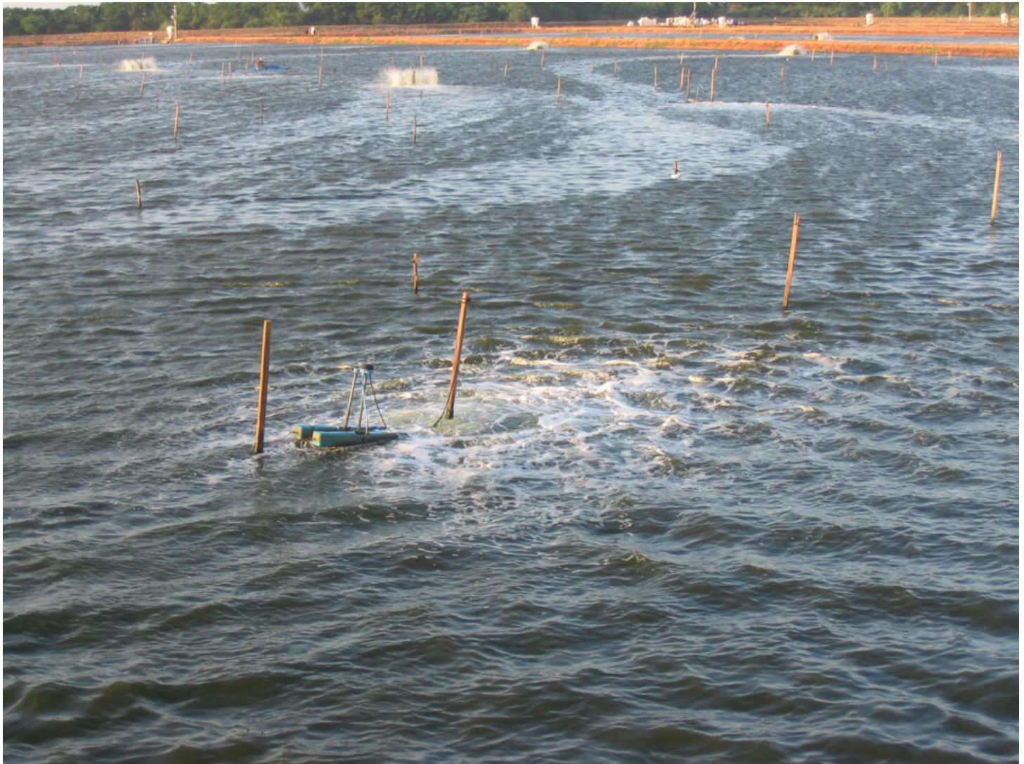
Mechanical aeration in ponds can prevent a deficit between net diffusion and net phytoplankton oxygen production. Photo by Darryl Jory.
