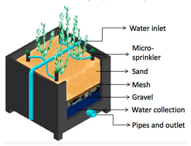
Fig. 1: The diagram shows the design of one lysimeter, depicting the overall construction, water inlet and outlet, substrate (sand and gravel separated by a mesh), and irrigation microsprinklers.
