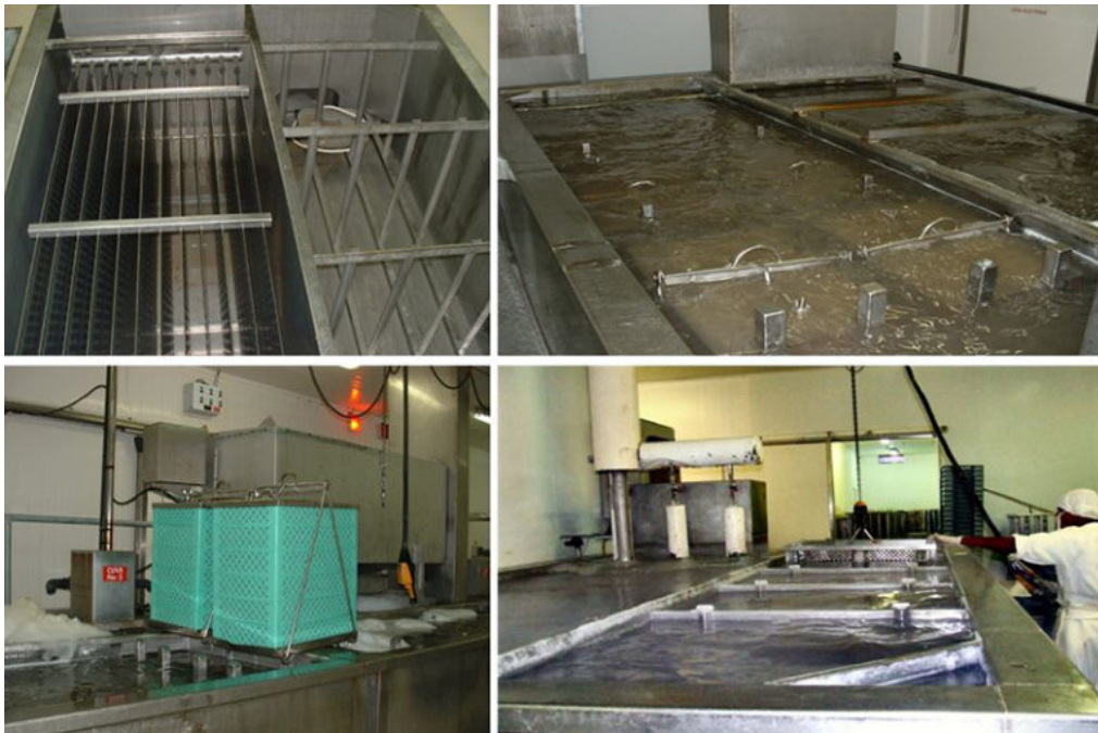
Views of empty and full brine freezers (top); dipping piles of shrimp blocks in brine freezing solution.
