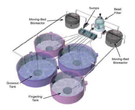
One possible layout for the fingerling/growout pods with common water treatment systems consisting of a propeller washed-bead filter and a moving-bed bioreactor. Illustration by Pradyot Deshpande.
