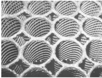
The biofilm established in the Bioblocks improves sedimentation by attracting small particles.
