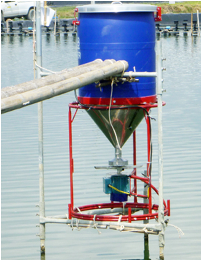
In small culture ponds, an automatic feeder can broadcast feed in a radius of 10 m and feed 600,000 shrimp. Timers control the broadcasting times and intervals of feeding.
