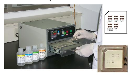
This mini hybridization oven was specially designed for multiviral biochip-based kits. The chip to right indicates the subject shrimp was infected with IHHNV and TSV.
